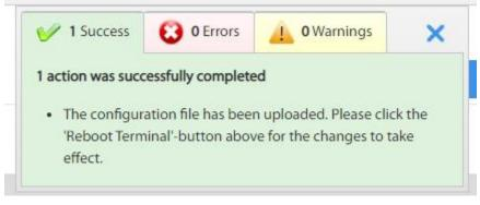
After both the package and options file have been loaded, click **Activate Software Package** for active1 or **Reboot Terminal**. Both will reboot the modem.
